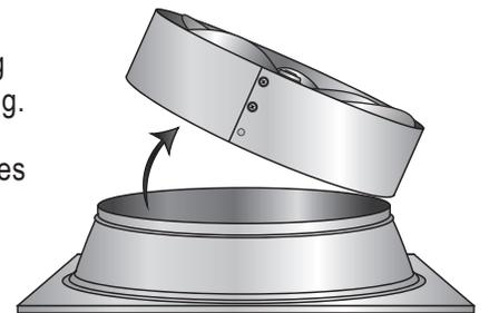
**Step 6:** Set Gable Ring on a flat surface with the fan facing up.
