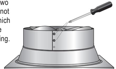
**Step 16:** Replace and tighten the four Gable Ring screws (in the 12, 3, 6, and 9 o'clock positions).
