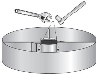
*NOTE: Observe how the old motor sits inside the bracket, and remove the old motor.*
