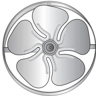
**Step 13:** Use the Allen wrench to tighten and secure the fan, leaving only 1/8" of the spindle showing above the hub.
