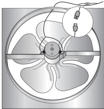
**Step 2:** After the fan blade stops spinning, disconnect the positive (red) wire and negative (black) wire from the motor.
