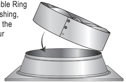
**Step 15:** Tighten the two screws (loosened but not removed in Step 4) which are found opposite the wiring on the Gable Ring.
