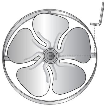
**Step 8:** Using a Crescent wrench and a Socket wrench, loosen (but don't remove) the two hex bolts on both sides of the motor bracket.
