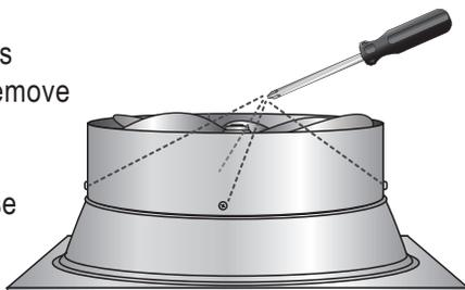
**Step 4:** Loosen but don't fully remove the two screws which are found opposite the wiring on the Gable Ring.
