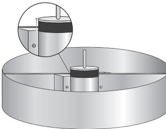
**Step 11:** Use the Crescent and Socket wrenches to retighten the two motor bracket bolts, so that the brackets are securely in contact with each other.
