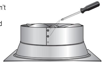
**Step 5:** Carefully remove the Gable Ring from the Gable Flashing.
