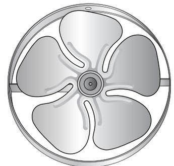
**Step 7:** Using the provided 1/8" Allen wrench, loosen the fan blade from the motor spindle, then remove the fan blade.
