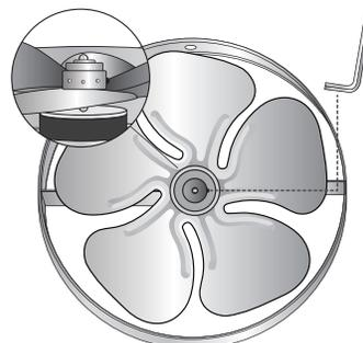
**Step 14:** Place the Gable Ring back on the Gable Flashing, being careful to match the hole pattern for the four screws.
