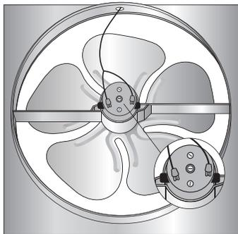
**Step 3:** Use the Phillips Head Screwdriver to remove the four screws (at the 12, 3, 6, and 9 o'clock positions) from the base of the Gable Ring.
